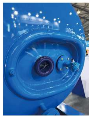
底部钽钉测温管 Bottom tantalum nail thermometer tube
